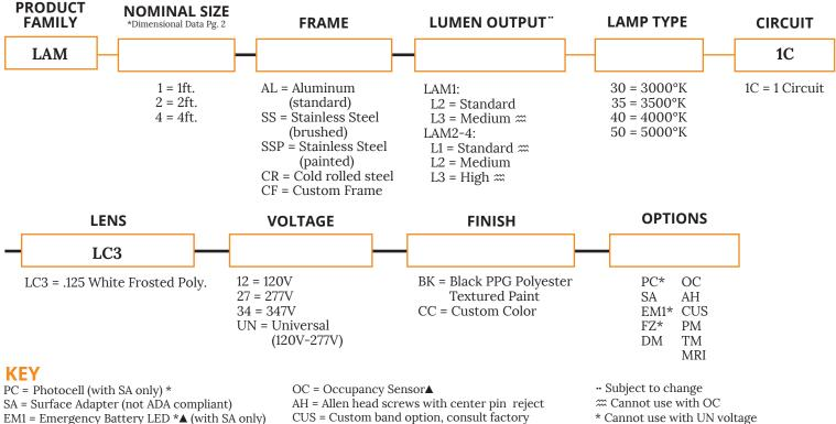
DM = 0-10V dimming with 10-100% range. Dimming wires will be extended outside of fixture (with SA only or L3)
