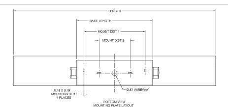
MOUNTING DIMENSIONS NOMINAL FIXTURE LENGTH MOUNT DIST 1 MOUNT DIST 2 LENGTH LENGTH HAV224 HAV248
