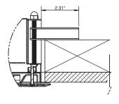
SCR (W/OC FRAME) RECESSED FLANGE
