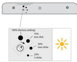
The LUMENSELECT® rotary switch should be turned gently clockwise with a small flathead screwdriver with a 1/8" or 3mm wide tip, one click at a time from factory setting to get desired output level.
