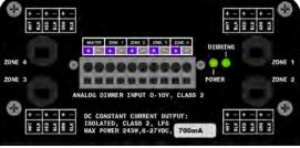
In MRI Installations, wall dimmers MUST be located outside the MRI room shield and must NOT be filtered.
