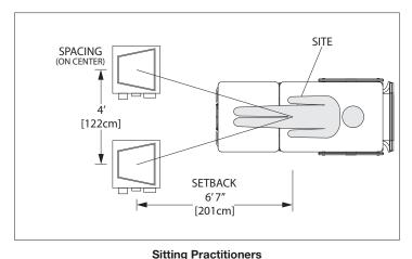
4' Spacing • 3' Work Plane • 53° Angle of Illumination
