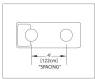
For optimal performance, fixtures should be placed 4' apart
