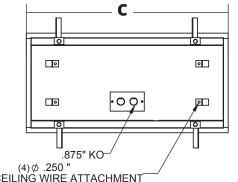
(4)  $\phi$  .250 " HOLES FOR CEILING WIRE ATTACHMENT
