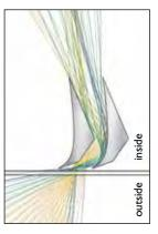
solar control. For all solar altitude angles, The patented LightLouver reflective slat design redirects daylight deep into the to provide uniform, glare-free daylight. daylit space while providing complete daylight up and back onto the ceiling LightLouver reflective slats redirect as shown in the diagram (left), the
